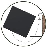
Align the groove above the bracket before lowering.
