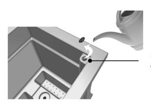
Remove fill port plug for direct access to the water reservoir.
