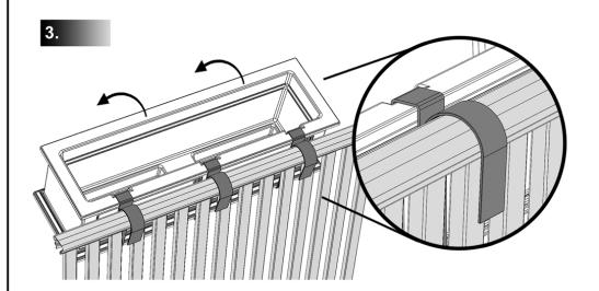
Hang the window box on the railing. Make sure the brackets fully slide over the handrail for a secure installation.
