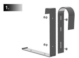
Align the handrail bracket with the wall mount brackets that shipped with your Mayne window box. For the Yorkshire window box align the bottom 2 slots on the deck rail bracket with the Yorkshire wall mount bracket. Fasten them together using the ½ Hex Bolt, ¼ Washer, and ¼ nut. Tighten firmly with a wrench.
