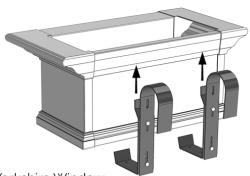
For the Yorkshire Window Boxes the brackets slide up into the groove on the back panel.
