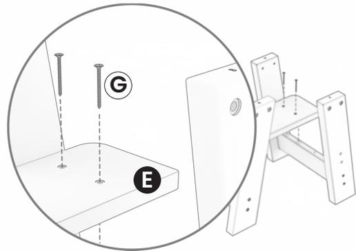
**5** Add the second shelf (**part E**) and secure it with 4 - M5x45mm wood screws (**part G**).
